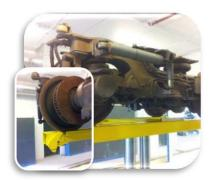
Each sole bar is equipped with two roll-off-devices. To assure highest possible safety, the roll-off-devices are monitored by integrated sensors.
