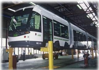
The tram is lifted via the bogie and is set down on the lifting columns. Every lifting column is equipped with a swivelling arm. If required, the bogie can be disconnected easily, can be lowered via the bogie lifters and new bogies can be mounted while the tram is held by the side lifters.
