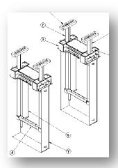
✓ Lifting capacity: 6.000 kg
