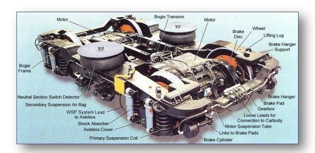
The bogie is the centrepiece of every rail vehicle where not only the wheels, brakes and suspensions, but also the complex drive train is situated. The unrestricted accessibility to all components which enable the quick and trouble-free maintenance is absolutely essential.
