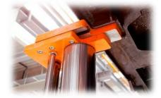
To assure that all gaps are closed at any time, the body lifting system is equipped with an aluminium-segment-cover with a capacity of 5 tons wheel-load. The sliding head-plate is equipped with a sensor, ensuring that it is always in the correct position.
