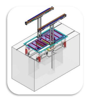
The synchronisation and redundancy of the left and right pistons is assured by a mechanical connection.
