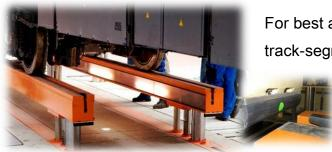
For best and safest working conditions, every track-segment is equipped with illumination,
