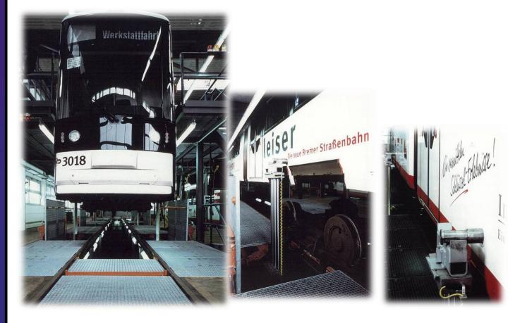
For this project the lifting units have directly been mounted on the bottom of a working pit.
