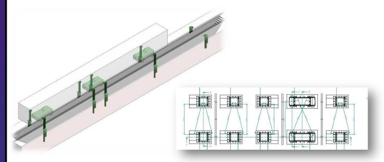
Exemplary view of customized lifting – system with stationary and moveable body-wok lifting units
