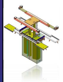
**d.)** This telescopic lift only requires an installation depth of approx. 1.300 mm.
