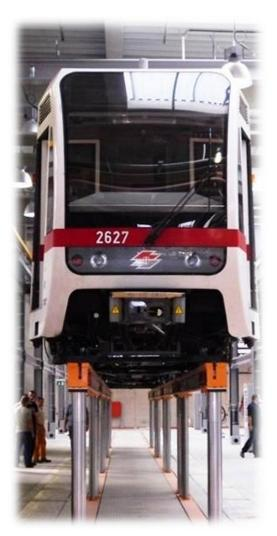
With its modular design, every GIANT consist of seven segments. Every segment comprises 4 track lifts, two (or four) moveable body lifting units and is controlled by an individual slave-control-unit. As a whole, each GIANT consist of 44 single rams, 7 Slave Control-units, 1 master control unit, 1 individually designed touch-screen panel, roof-working spaces and spans over a length of more than 40 m, offering a total lifting capacity of more than 150.000 kg
