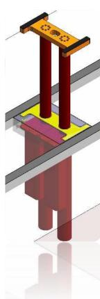
Every lifting unit consists of two hydraulic cylinders and one head-plate.
